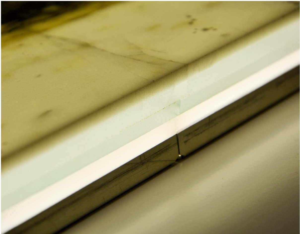
Marble backlighted with more LED light panels. Translucency is homogenous.
